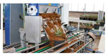
Easy change over is therefore possible. Because of the spinning and the sweeper at the end of the line, a uniform covering result is achieved. The excess material that falls beside and off the pot will fall back in the main hopper and is re-used.
