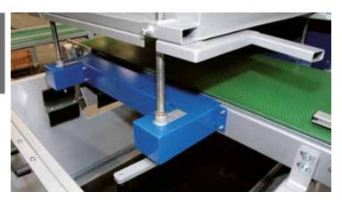
of the rotor and the height of the filling head the soil density can be adjusted. An optional soil recycling system is mounted at the end of the filler to collect the access soil and to bring it back to the soil hopper for reuse.
