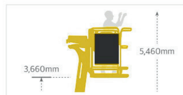
Max. ascending height of the working plate & Max. height available for work
